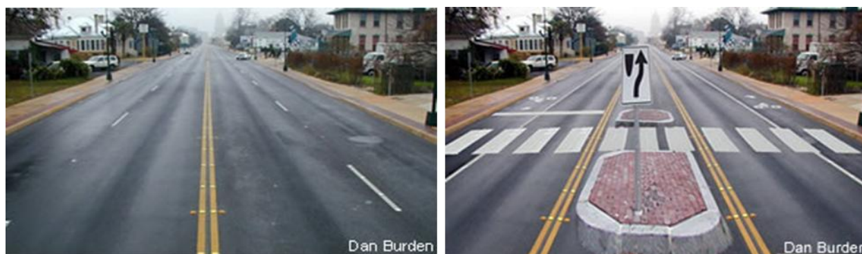
The classic road diet converts a four lane section to three lanes. In this scenario, the bike lane provides a buffer to pedestrians walking on the sidewalk adjacent to the curb.
